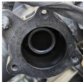
Where the diverter valve mount has metal threaded inserts as shown below, use the supplied fine-pitch screws (requires a 5mm hex key). Tighten to 6-8Nm (4.4-6lbf-ft).
