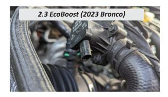
1) Remove the electrical connector from the factory diverter valve. First slide the grey locking tab out, then push it down to unclip the connector:
